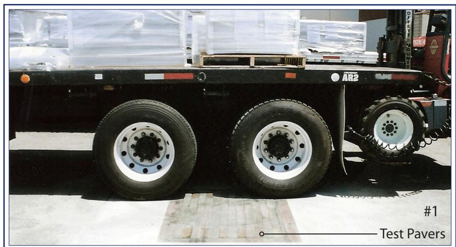
placement of the Narrow Modular Paving units. Setting the pavers in mortar was followed by the mandatory placement of the joint sand and stabilizing material. The test area was
