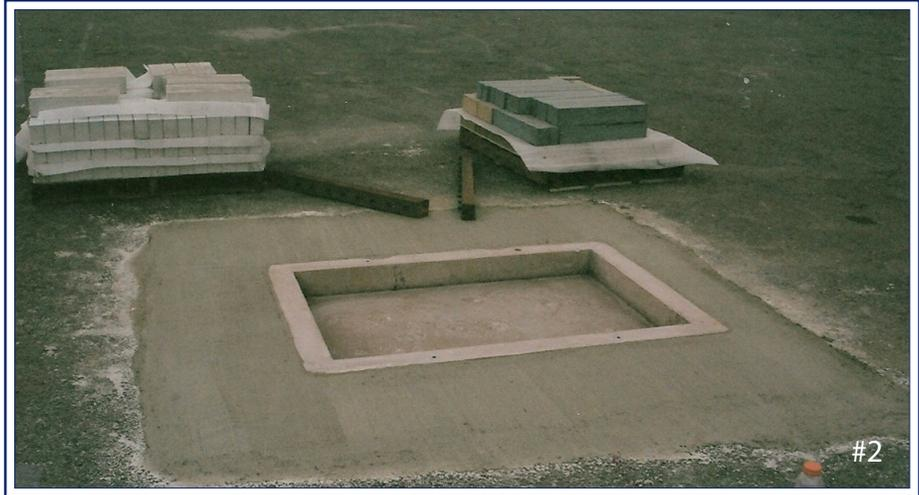
A precast slab with four-5" thick containment walls was placed in the asphalt parking lot. The paving area was 36½" x 54". The slab below the pavers was four inches thick.
